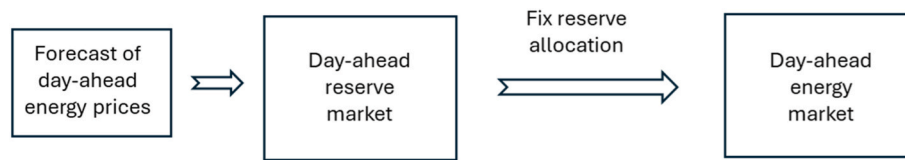
Fig. 2. Graphical representation of the modeling implementation of the (Seq) design which we use for efficiency benchmarking of the IPTO proposal for the Greek market.
