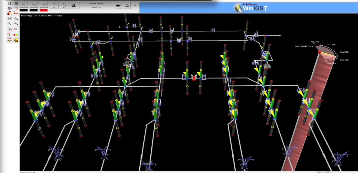
Example Visualization Substation Operating Conditions
