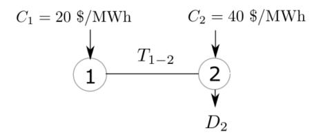
Suppose  $D_2 = 50 \text{ MW}$ ,  $T_{1-2} = 50 \text{ MW}$
