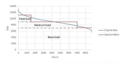
**Load duration curve** is obtained by sorting load time series in descending order
