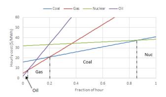
**Screening curve**: Total hourly cost as a function of the fraction of time that a technology is producing
