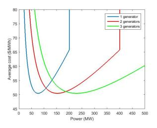
Average cost at unit capacity (200 - 220 MW) is lower for n=3 generators
