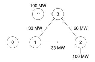
Figure: A 4-node network with no passive element connected to ground can be represented as a 3-node network by ignoring the ground node.
