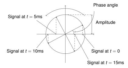
AC power systems have voltage and current that fluctuate sinusoidally (50 Hz in Europe, 60 Hz in USA)
