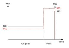
Figure: Demand under fixed retail pricing (black solid curve) and time of use pricing (red dashed curve). Effect of ToU pricing: depresses consumption in peak hours, increases consumption in off-peak hours.
